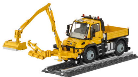
UNIMOG U430 ROAD/RAIL VEHICLE WITH COMBINATION MOWING IMPLEMENT
